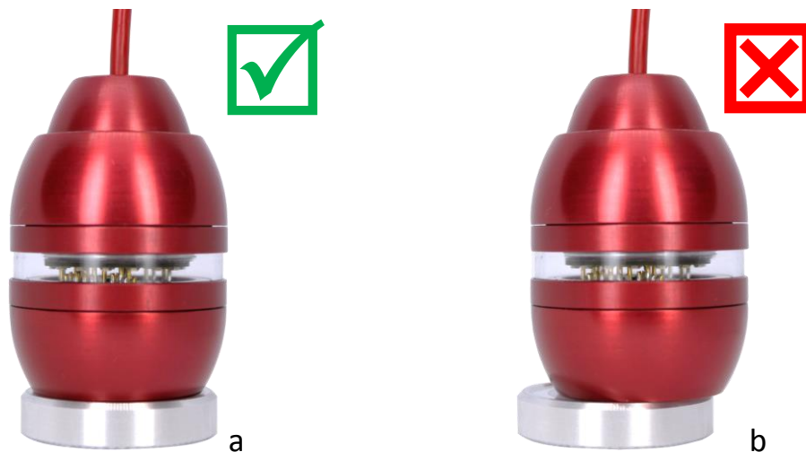
Fig. 4. Minispectrometer orientation relative to the etalon at calibration measurement: a – correct, b - incorrect.
