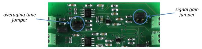
**Note!** To find out more about mode adjustment of the synchronous detector please refer to the SDM synchronous detector manual.
